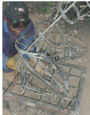
Fig 8: Joining rings to the spine
