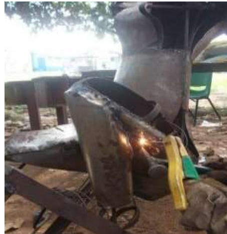
Figure 18: Forming and joining the thigh.
