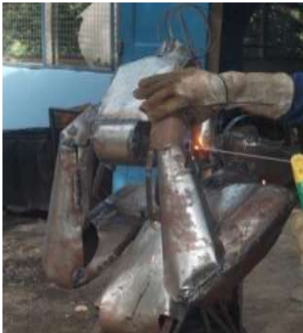
Figure 17: Welding the lower arm:
