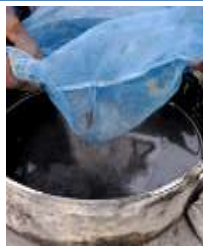
Fig.10.3 sifting charcoal with seive Fig.10.4 charcoal mixed with water. Fig. 10.5 charcoal, clay and water
