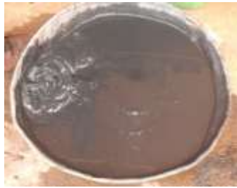
Figure 10.8 prepared slurry for the second coating
