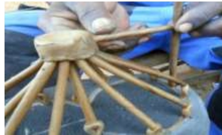
Fig 12.2 Softening sprues using heat Fig. 12.3 making gates and air vents Fig. 12.4 Complete structure.
