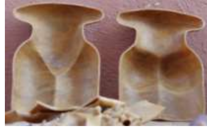
Figure 9.9; splitted wax modle
