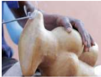
Figure 10.0; welding detouched wax modle together
