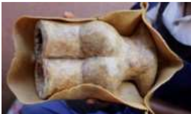
Figure 9.4; pattern being wrapped with wax sheet
