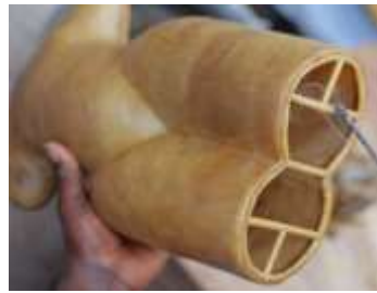
Figure 10.1 tacking the modle with wax rods
