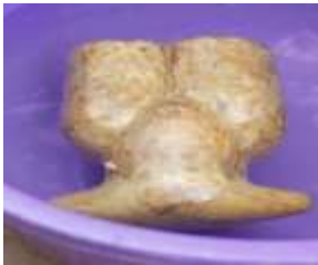
Figure 9.2; pattern being hardened in cool water
