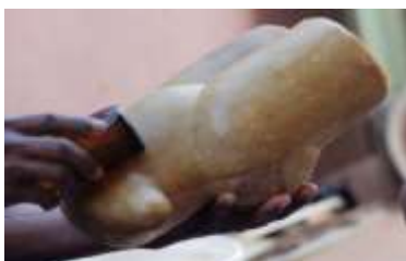
Figure 9.6; smoothing wax sheet on pattern
