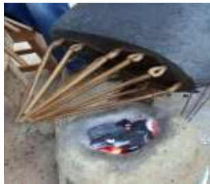
Fig 12.2 Softening sprues using heat Fig. 12.3 making gates and air vents Fig. 12.4 Complete structure.
