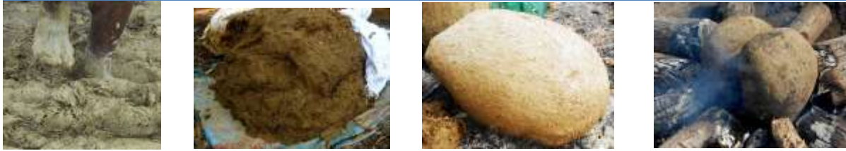
Fig. 12.5 coating mixture. Fig. 12.6 mixture preparation. Fig. 12.8 Complete Mould. Fig.12.9 Dewaxing
