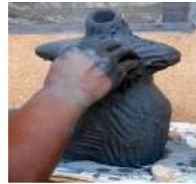
Figure 10.9 first stage of the second coating
