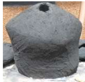
Figure 11.2 fourth stage of second coating
