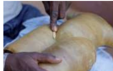
Figure 9.5; dressing wax sheet around pattern
